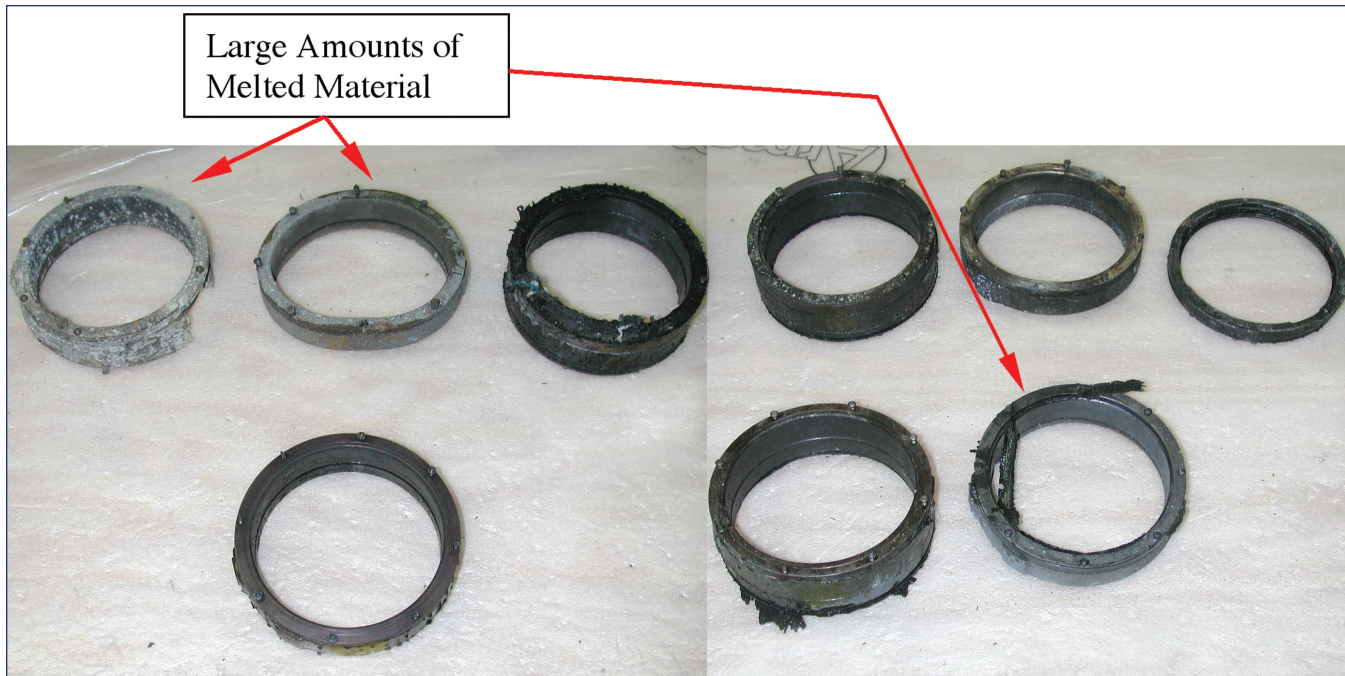
Recovered Glove Disconnects.
